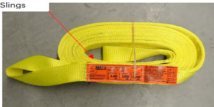
Identifiable markings on Synthetic Slings
