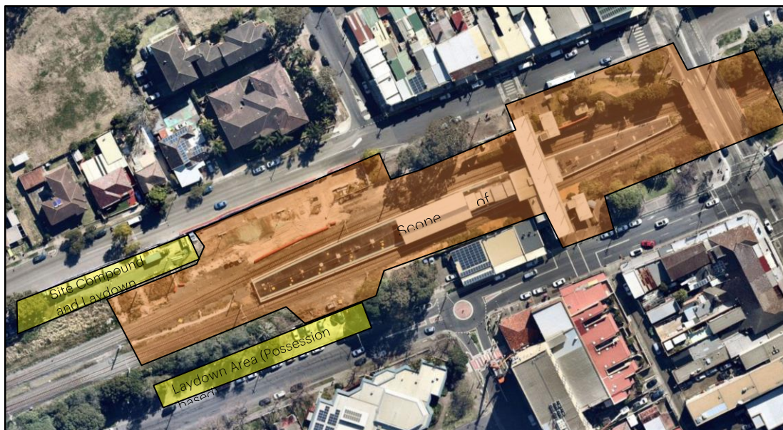
Figure 4 – Lakemba Station – i) Scope of Works Area, ii) Site Compound and Laydown Area and iii) Laydown Area (Possession based)
